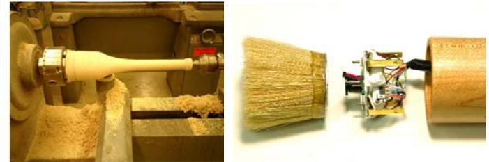
**Figure 6.** The brush handle on a lathe (left) and the video camera and components inside the brush (right).
